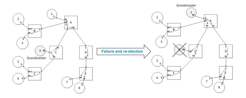
The clock synchronization protocol is a classical master-slave protocol. The master is called the "grandmaster".
